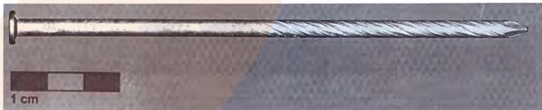
tested nail 4,60 x 145 mm spiral HDG
