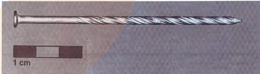
tested nail 3,40 x 100 mm spiral HDG
