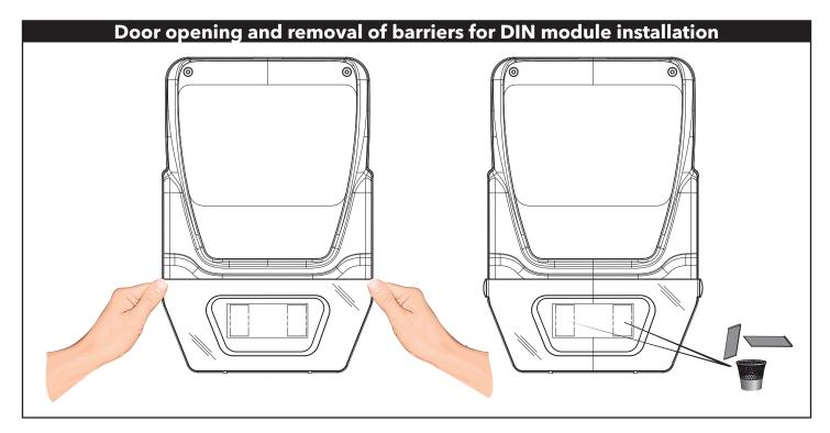
The versions with front door allow direct access to the switch miniature circuit breaker or to the top of the device installed on the DIN rail mounted inside.
