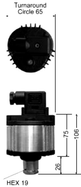
Figure 6: Pressure Connection: Style 47 (Dimensions in mm)
