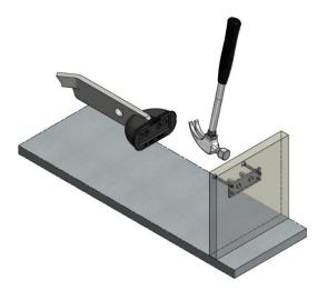
Nail or screw the TMP product to the wooden formwork and press the RBF with the anchor inserted into the holding plate.
