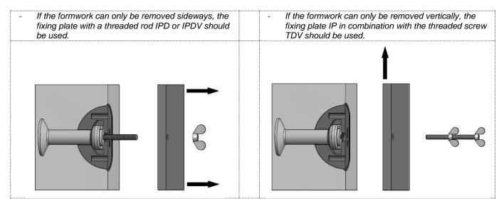
The fixing plate with a threaded rod IPD or IPDV and the anchor are fitted in the opened recess former. The recess former is mounted to the formwork with the wing nut. The nut is then tightened securing the recess former and the anchor firmly in position.
