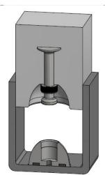
When using this magnetic recess former, it is very important that the surface of the formwork is clean. After demoulding, the magnetic former can be removed from the formwork with a screw.
