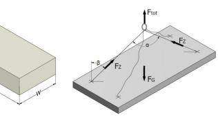
The slab unit has the following dimensions: L = 5 m w = 2 mt = 0.2 m
