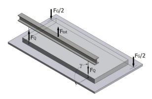
The slab unit has the following dimensions: L = 7.5 m w = 2 mt = 0.18 m
