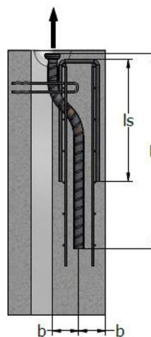
**Using an additional sandwich hairpin anchor installed near the anchor is beneficial.**
