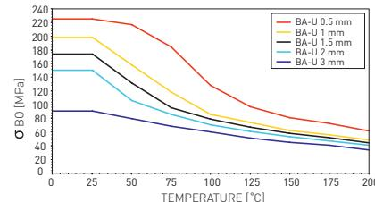
σ<sub>BO</sub> diagrams represent σ<sub>BO</sub> values for different gasket material thicknesses. These values indicate the maximum in-service compressive pressures which can be applied on the compressed gasket area in-service without destroying the gasket material.
